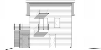
5 CARRIAGE HOUSE A - NORTH ELEVATION 1/8" = 1'-0"
