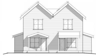
4 DUPLEX BB - FRONT ELEVATION 1/8" = 1'-0"
