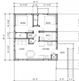
2 CARRIAGE HOUSE A - LEVEL 2 1/8" = 1'-0" UNIT AREA - 624 SF
