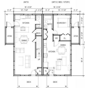
1 DUPLEX BE - LEVEL 1 1/8" = 1'-0" UNIT B AREA: 861 SF TOTAL SF UNIT E: 960 SF
