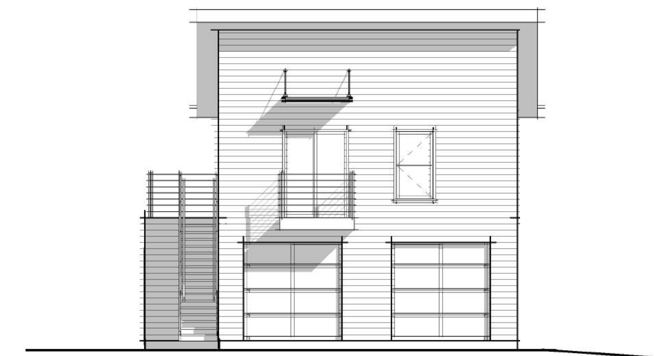
5 CARRIAGE HOUSE A2 - NORTH ELEVATION 1/8" = 1'-0"
