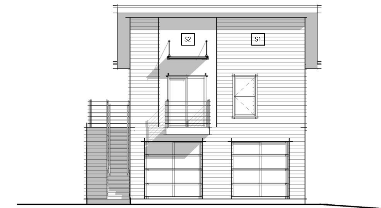
5 CARRIAGE HOUSE A2 - NORTH ELEVATION 1/8" = 1'-0"
